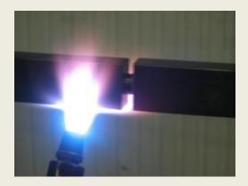
Occasionally, the conductor has to be spliced. A tough bit of plumbing. Without good quality control in the brazing, the joints would leak when warm and pressurized.
