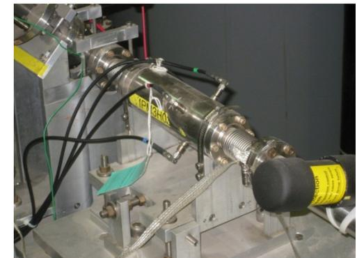
Generic example of beam modulation and measurement system that has been used for many of these experiments - capability to measure helicity correlated beam properties continuously and deliberately vary beam position, angle and energy.
