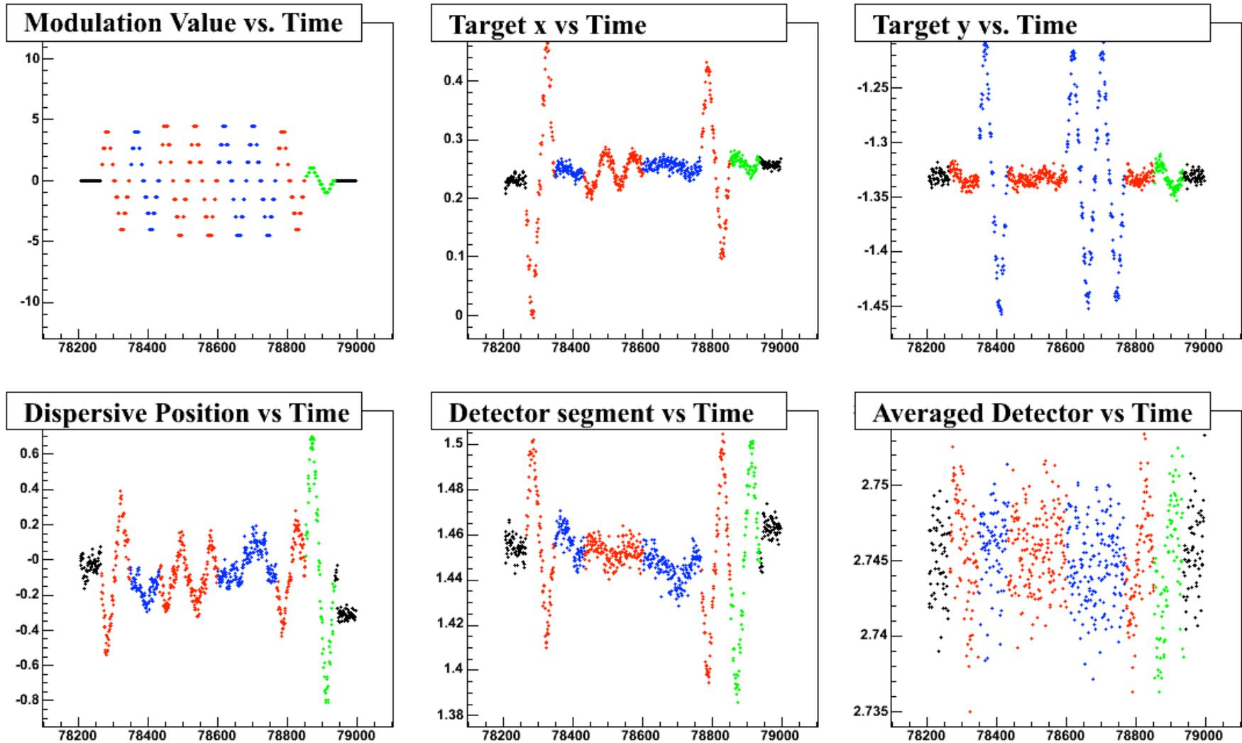
HAPPEX coil dithering system previously used in Hall A; uses 7 air-core coils and energy vernier with a single modulation cycle (represented above) lasting 23 seconds.
