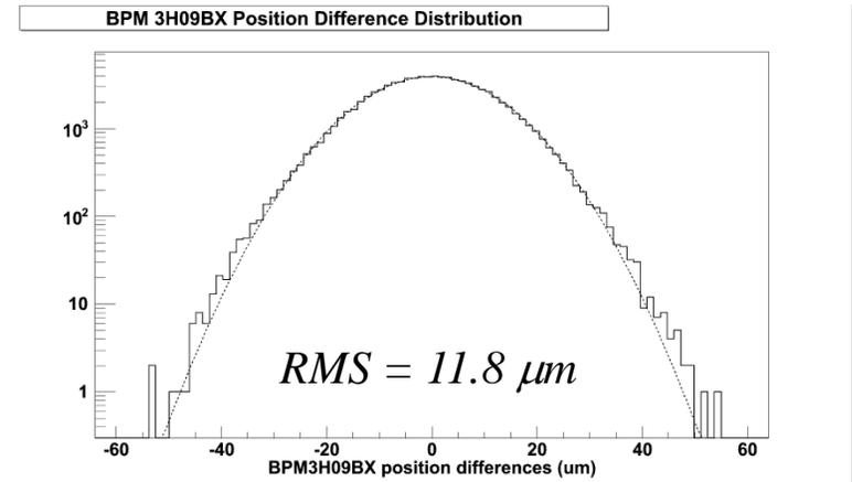
Measured vs. projected position at BPM3H09X
