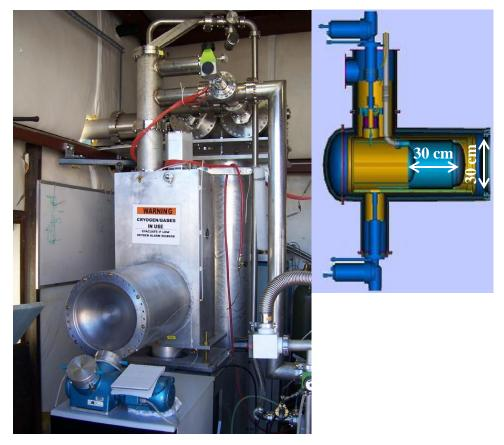
20L vessel of liquid parahydrogen
