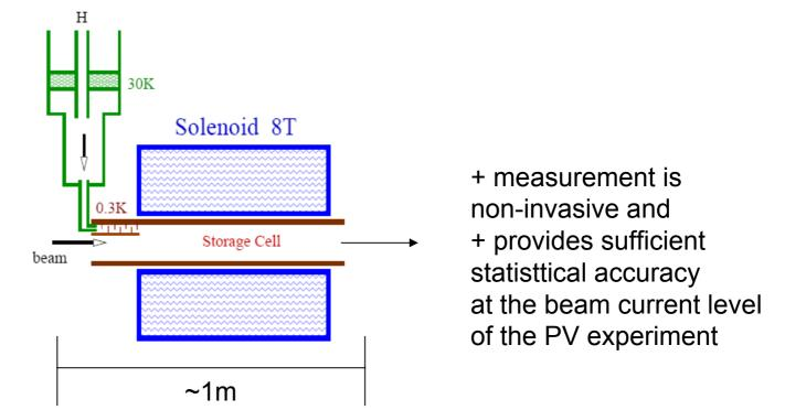
Solenoid traps pure H<sup>↑</sup> which has a long lifetime due to He-coating of storage cell. All other species are removed quickly from the trap.  $\rightarrow$ 1- $\epsilon$  Polarization can be reasonably well estimated, but measurement difficult.
