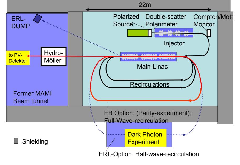
"Unimpeachable" polarization measurement: two independent polarimeters with  $\Delta P/P < 0.5\%$  (NOT: 1%) each.
