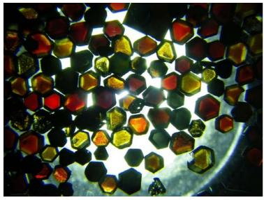
Color: NV-centers introduced in Diamond. Irradiated at MAMI for 3 days,  $50\mu$ A at 14MeV (J. Tisler et al. ACS NANO 3,7 p.1959 (2009))
