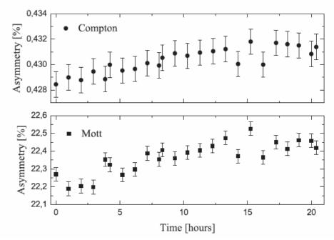
Polarization Drift consistently observed in transverse AND longitudinal observable at the <0.5% level (Measurement at 3.5 MeV, 35  $\mu$ A) Compton is an analogue, Mott a counting measurement
