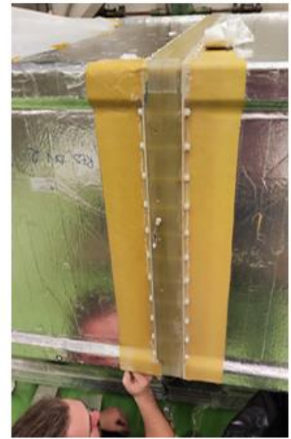
High Voltage feedthrough external connection
