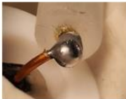
High Voltage feedthrough external connection
