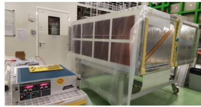
High voltage tests after assembly
