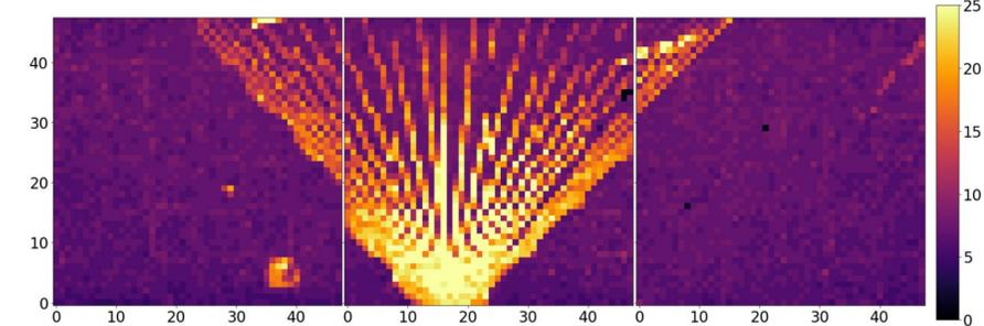
Example of a series laser shot fired at different azimuth angle, detected during the field campaign of EUSO-SPB2 in 2022. The laser was fired from 28 km away, pointing at 45° zenith angle. The bright spot is due to a lamp in the field of view of the instrument
