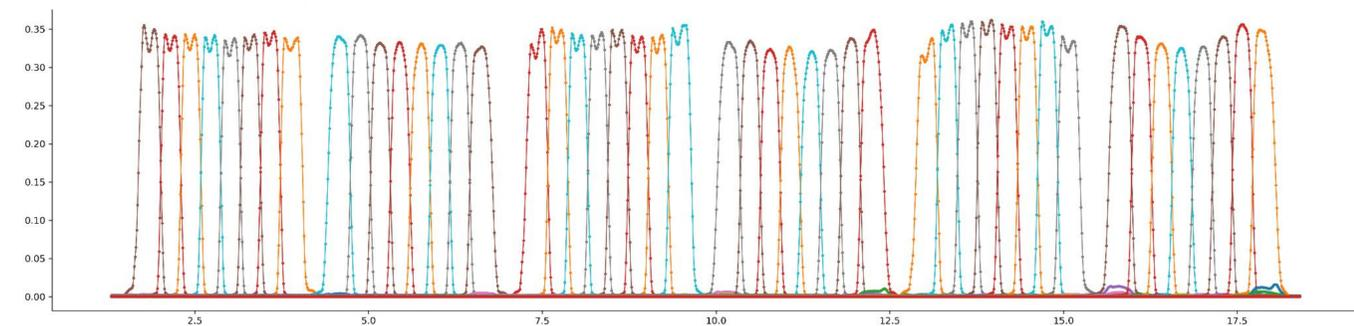
Scan across an EUSO-SPB2 PDM, showing the response of all pixels to local illumination, namely the photodetection efficiency (in percent), as a function of position (in centimeters). Details of the internal structure of the MAPMTs are visible
