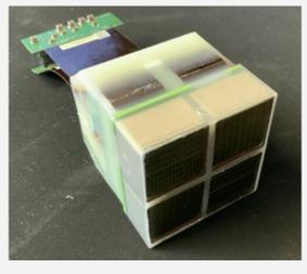
A packaged Elementary Cell (EC). All the electronic components are hosted in the shadow of the 4 MAPMTs.
