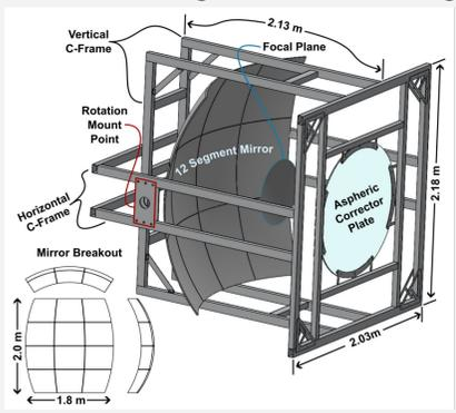
Design of the tiltable frame that host the optic system and the FC and CC focal planes.
