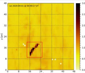
Example of a meteor observed by the Mini-EUSO detector looking nadir from the ISS
