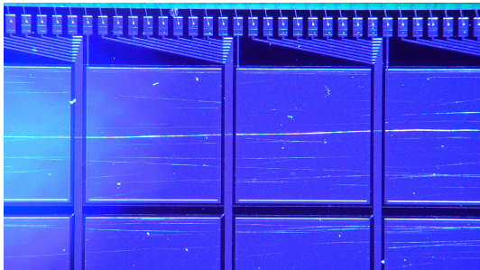
Gallium Arsenide sensor with traces in the sensor
