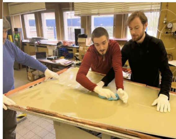
Leak test (drop < 0.4 mbar/10 min)
