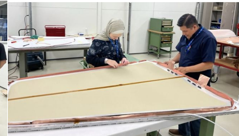
Dark current test (< 2.5 \mu A)
