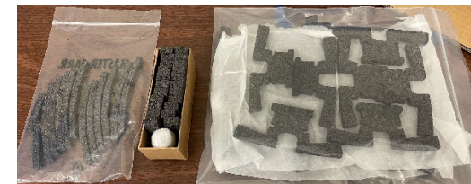
Carbon foam layer 3 end ring pieces
