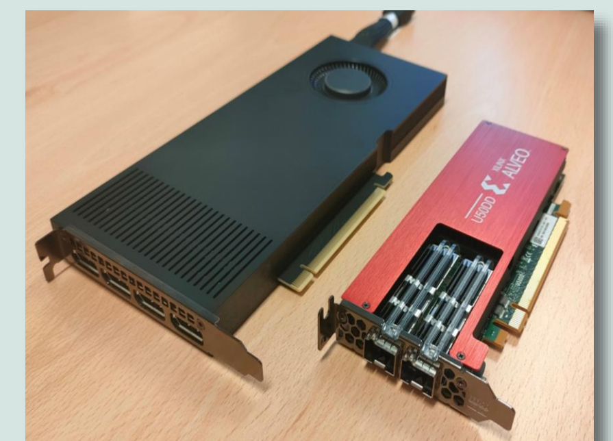
Fig.6 - Used GPU and FPGA modules
