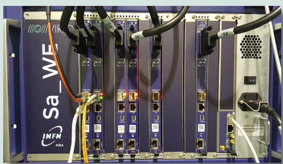
Fig.1 - MTCA (custom) based crate used in AdV+ control electronics
