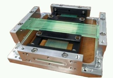
Single X-Y module: 3 mm thick LYSO crystal coupled with two crossed planes of Kuraray Y-11 1 mm square WLS fibers, on its top and bottom faces. The fibers are read-out by a Hamamatsu 128channels SiPM array S13552.
