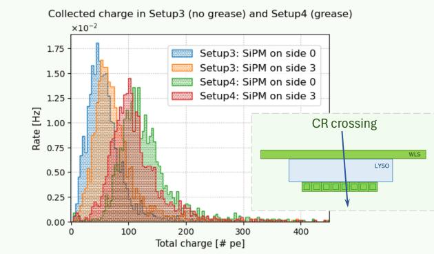
Setup3 vs Setup4 - CR: more light is collected in the Setup4 thanks to the optical grease between the WLS fibers and the LYSO crystal.
