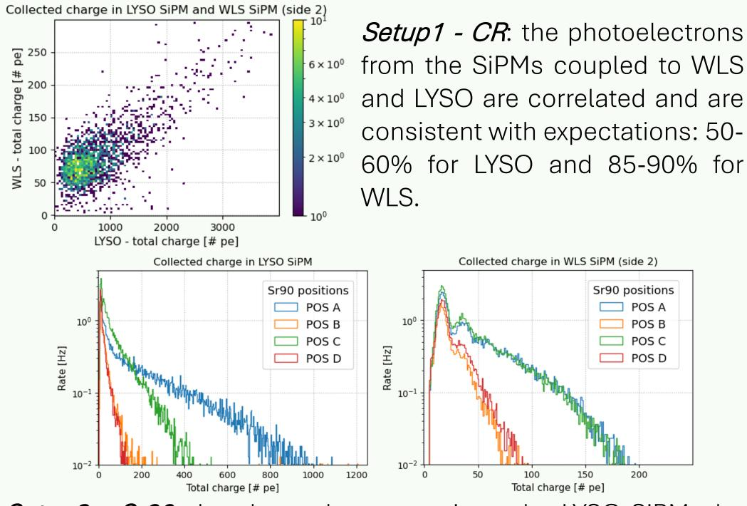
Setup1 - CR: the photoelectrons from the SiPMs coupled to WLS and LYSO are correlated and are consistent with expectations: 50-
