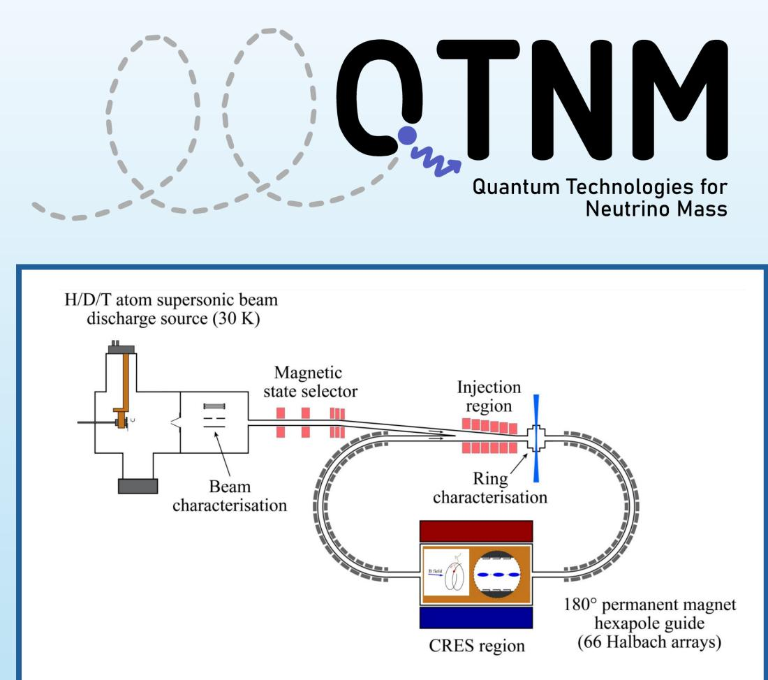
Cyclotron Radiation Emission Spectroscopy (CRES) is a method for measuring the kinetic energy of an electron undergoing cyclotron motion in a magnetic field. The frequency of the radiation is directly linked to the magnetic field and kinetic energy of the electron by
