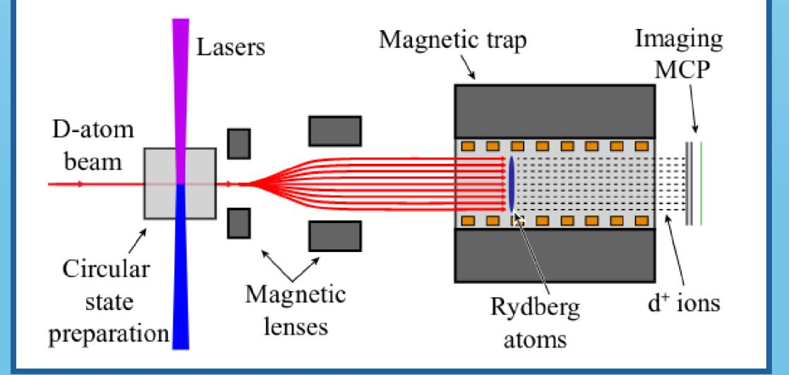
For beta decay to occur, it is necessary to keep atoms in the detection region. A storage ring can provide good timeaveraged density of atoms in the detection region by guiding atoms using magnetic fields.
