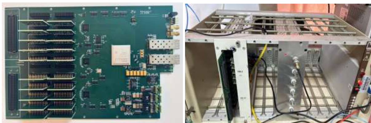
Figure 11 readout electronics(Each NIM accommodates 3 readout boards and 1 High voltage board)
