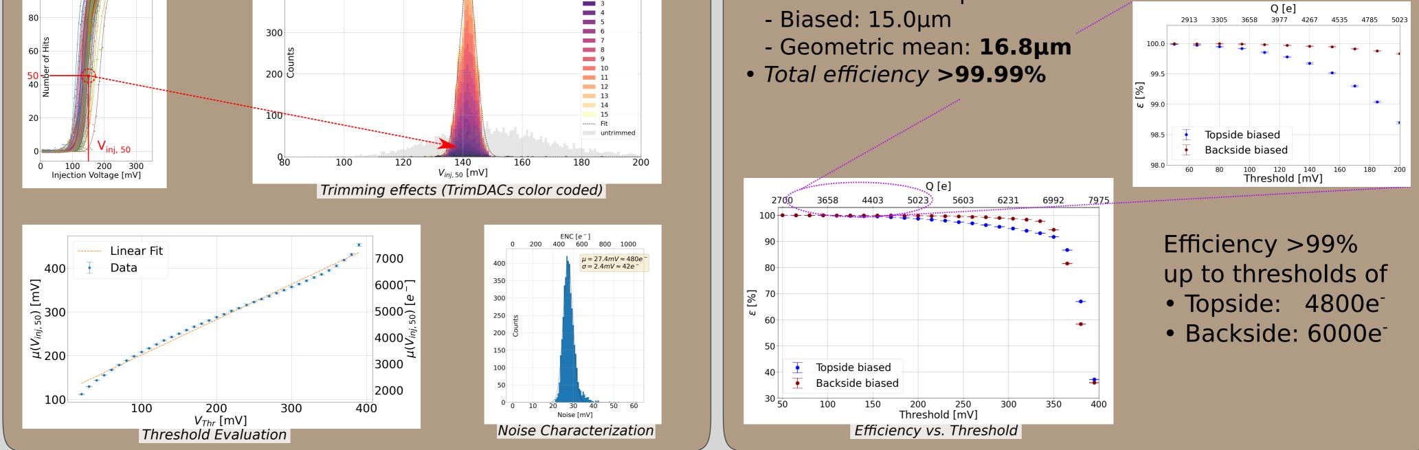
Finding and fixing the problems of RD50-MPW3 lead to the development of the **RD50-MPW4**. This protype was successfully characterized in the laboratory and at beam tests. Summary The measurements show a high breakdown voltage of a few 100V, a uniform pixel response ( $\sigma \approx 50e$ -), a spatial resolution of  $\approx 17 \mu m$  and an efficiency >99.99%.
