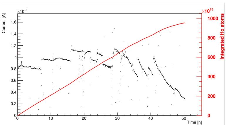
Extraction efficiency evaluated using <sup>165</sup>Ho, by acquiring long run ( $\sim$  50 h) up to a total consumption of a target, then comparing the integrated charge w.r.t. the <sup>165</sup>Ho content in target.  $\varepsilon \sim 0.2$  %, enough to proceed to first implant.
