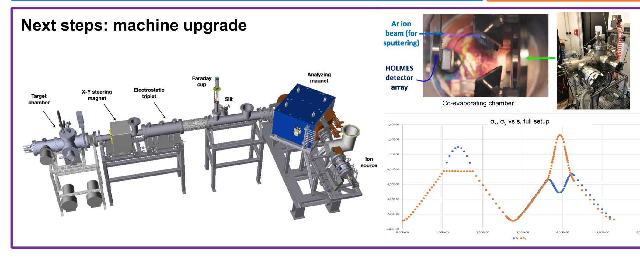
To increase the maximum achievable activity and obtain a more effective beam handling, an upgrade of the beam line is currently on going. The setup will be extended by adding a quadrupole triplet, a x-y steering magnet and a target chamber to allow co-evaporation of Au during Ho implantation. With this configuration we expect to be able to get a beam size of  $\sigma \sim 1.1$  mm.
