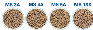
Crystalline metal aluminosilicates having a three-dimensional interconnecting network of silica and alumina tetrahedra
