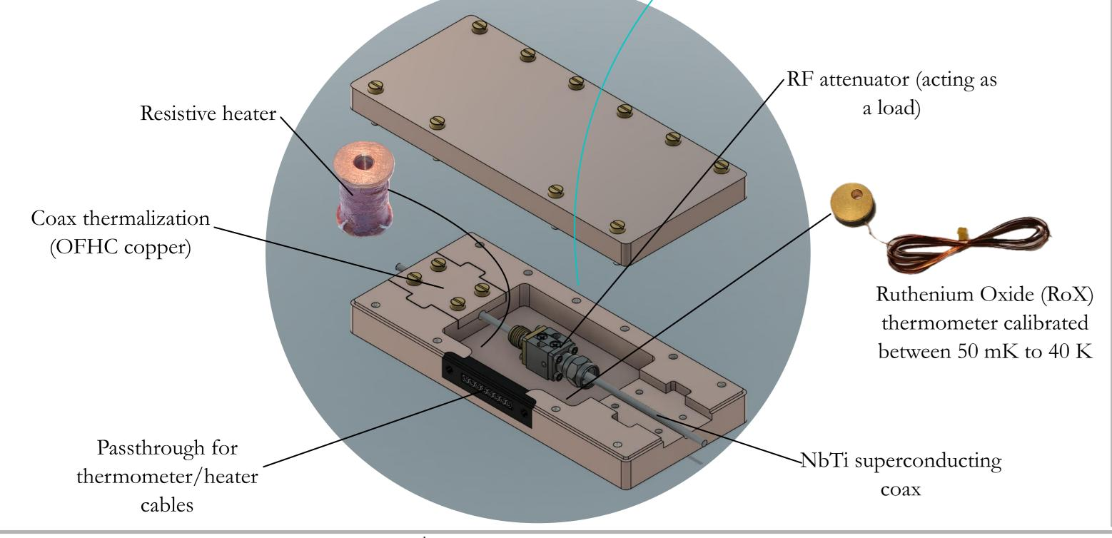
to measure the noise with the Y-factor method in principle only two temperatures are required
