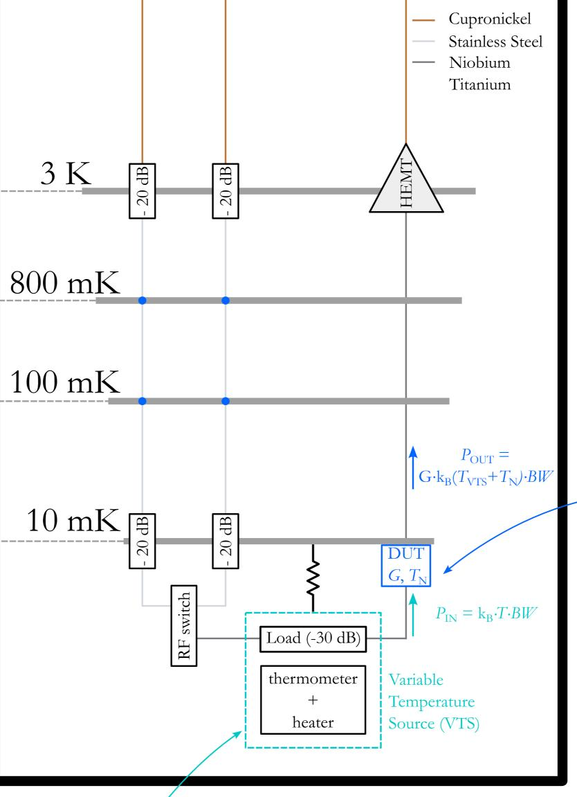
the DUT is a low-temperature, low-noise amplifier, such as Traveling Wave Parametric Amplifiers (TWPA), such as the ones developed within DARTWARS (see A. Giachero's talk on Thursday 9:10 a.m.)
