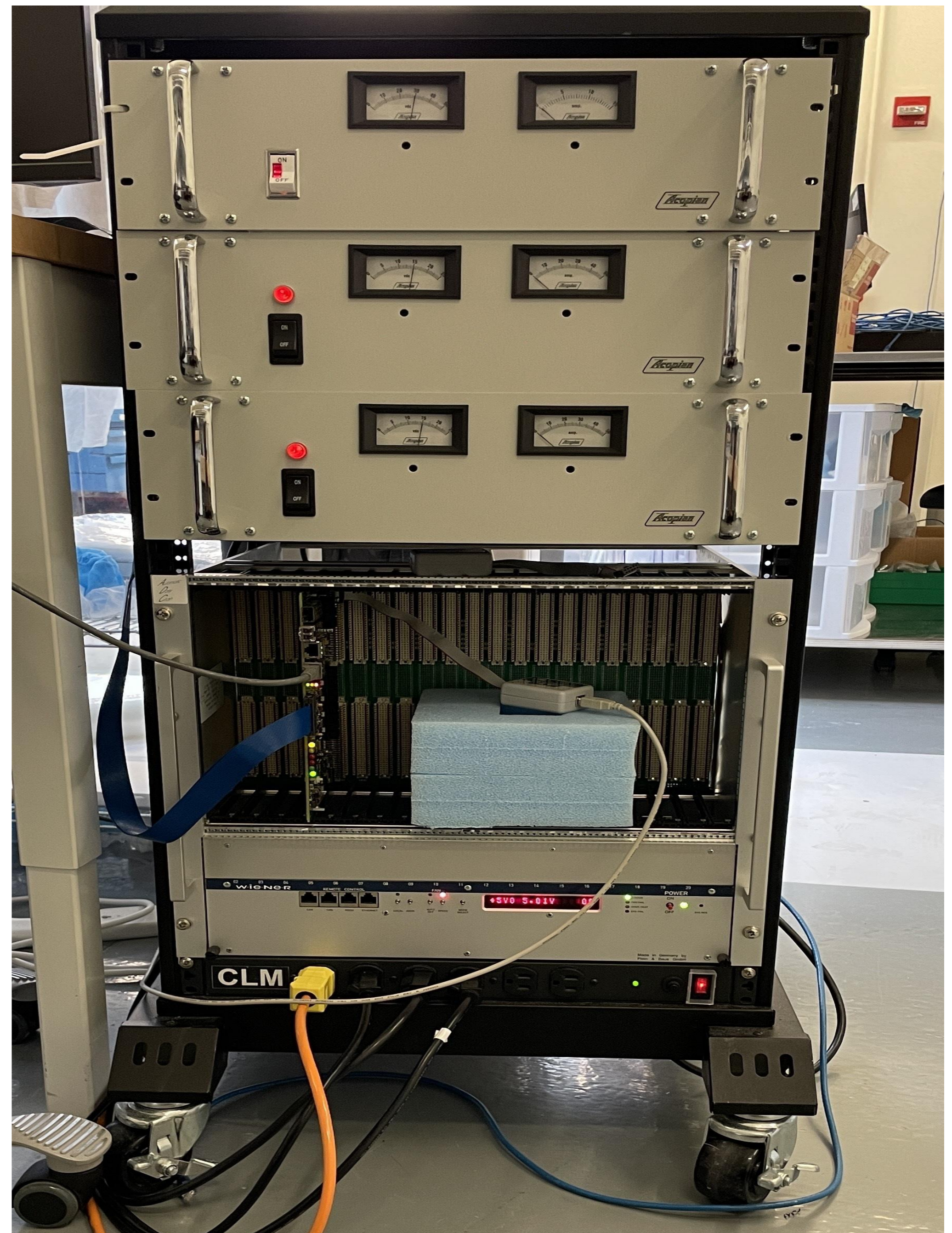
Figure 2. Prototype ACM board inside VME crate with linear power supplies.
