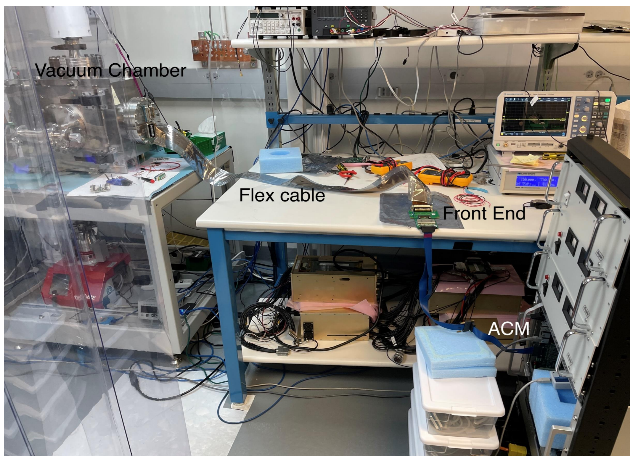
Figure 1. CCD control and readout electronic chain.
