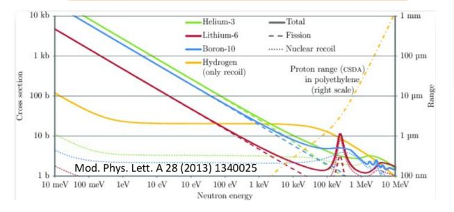
Thermal neutron detection relies on the neutron capture and thus conversion to ionizing particle: <sup>3</sup>He shortage  $\rightarrow$  <sup>10</sup>**B** alternative: <sup>10</sup>**B**<sub>4</sub>**C converter**.
