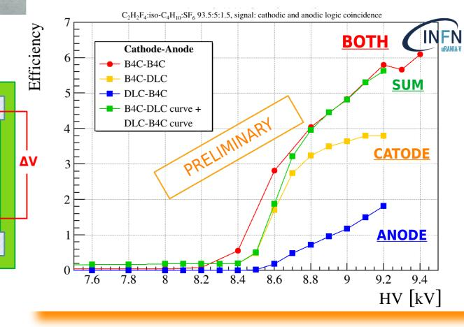
$\alpha$ /<sup>7</sup>Li **mean path** < **2mm**  $\Rightarrow$  CAT and AN have different behaviors • <sup>10</sup>B<sub>4</sub>C CAT – **DLC AN** : the expected 4% plateau was reached • **DLC CAT** – <sup>10</sup>**B**<sub>4</sub>**C AN** : efficiency depends on the HV •  ${}^{10}B_4C CAT - {}^{10}B_4C AN$  : the  ${}^{10}B_4C - {}^{10}B_4C$  performs as the SUM
