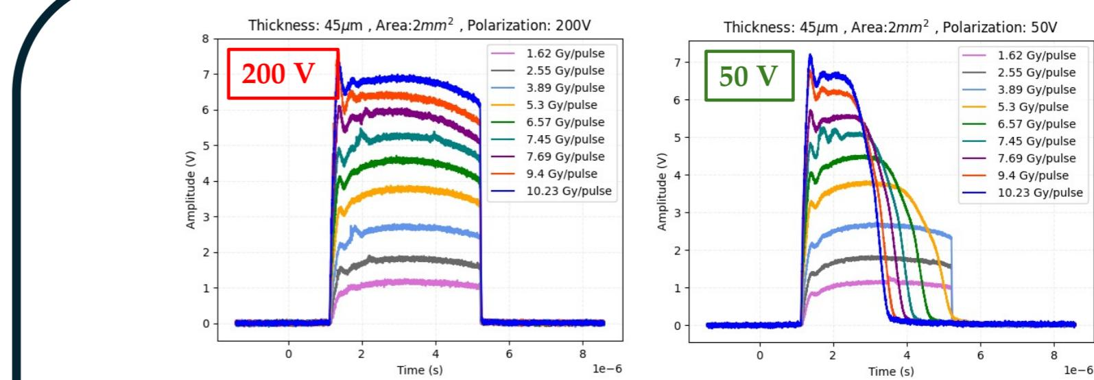
High density of charge carriers generates an opposing electric field that cancels the drift field, inhibiting charge collection.
