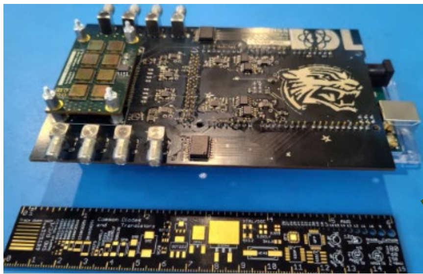
Figure 2b) Validation boards for the analog front-end design for the TIGERISS photo-detector modules. Constructed at Penn State, this large form factor unit is being tested currently to evaluate the SiPM performance.
