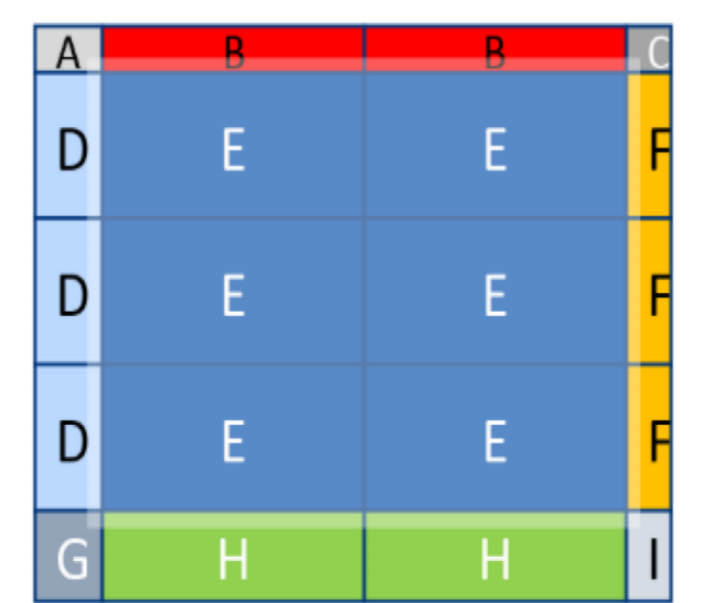
Figure 3: ULTRASAT sensor stitching diagram: A,B,C,F,I - seal rings; D - Row Decoders; E - Pixel array; G - digital block; H - ADC
