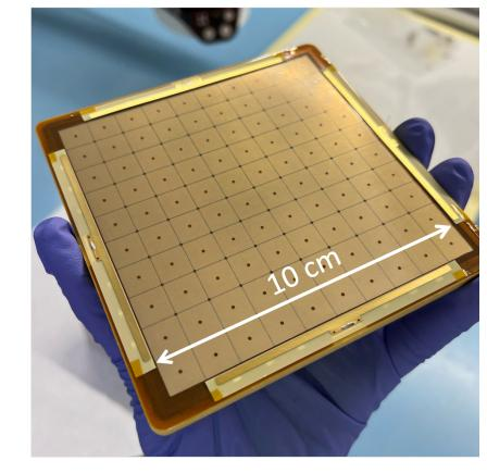
100-channel module Single-pad prototype
