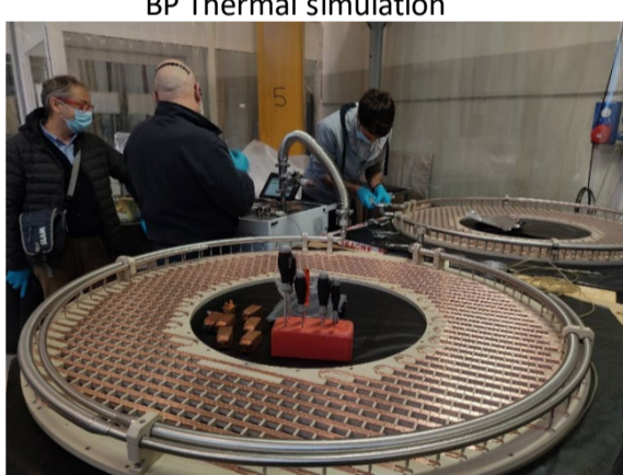
BP leak tests
