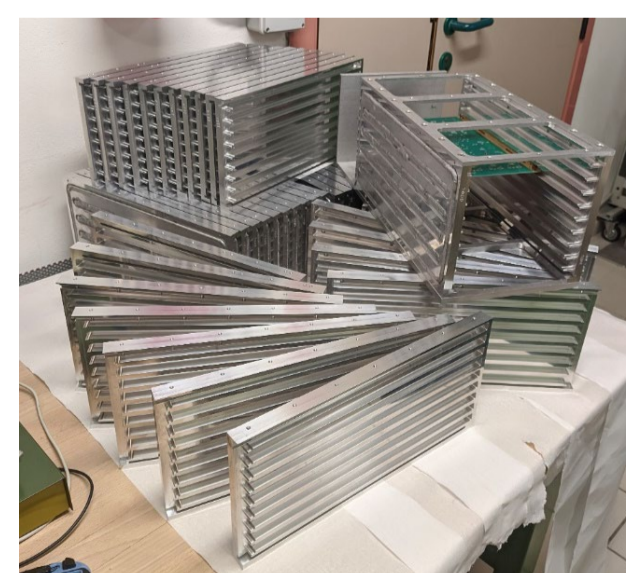
Crate sides during leak test
