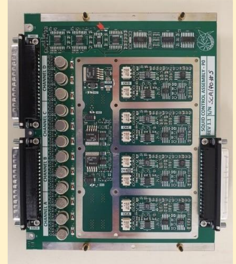
The SQUID Control Assembly (SCA) board, each of these controls 4 SQUIDs.
