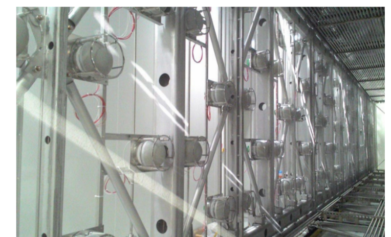
360 HAMAMATSU R5912-MOD (8" diameter) PMTs mounted behind the TPC wire planes.
