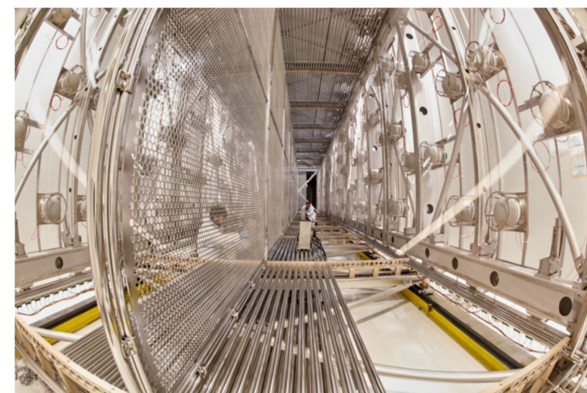
360 HAMAMATSU R5912-MOD (8" diameter) PMTs mounted behind the TPC wire planes.
