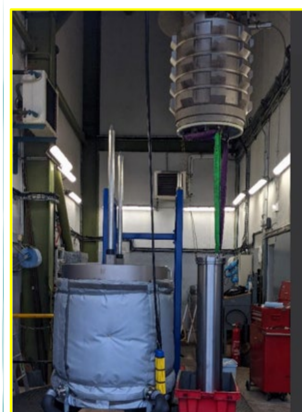
BM titanium container ready to be moved in the hyperbaric chamber at IFREMER, France
