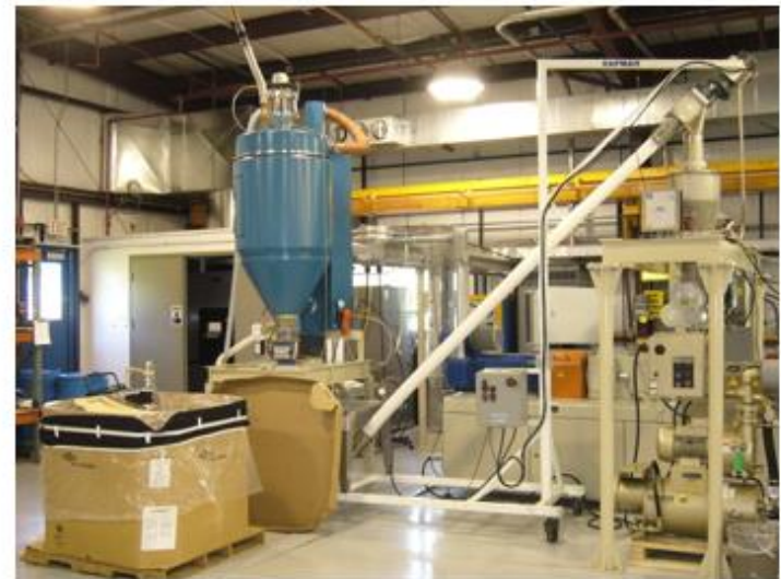
Head of system showing dryer, extruder, and cladding co-extruder
