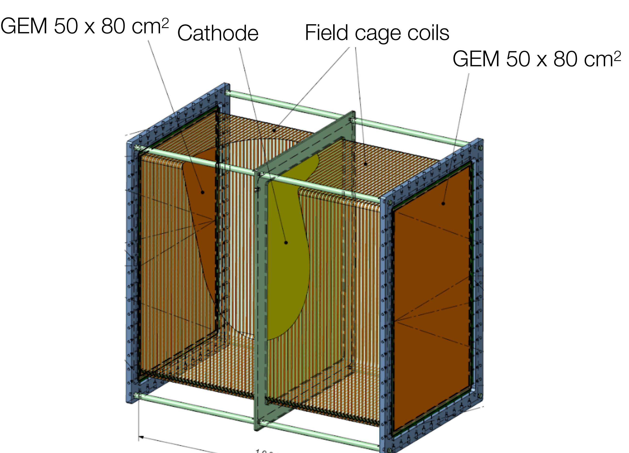
**CYGNO\_30:** O(30 - 100 m<sup>3</sup>) detector for directional DM searches in the ~GeV/c<sup>2</sup> mass region.
