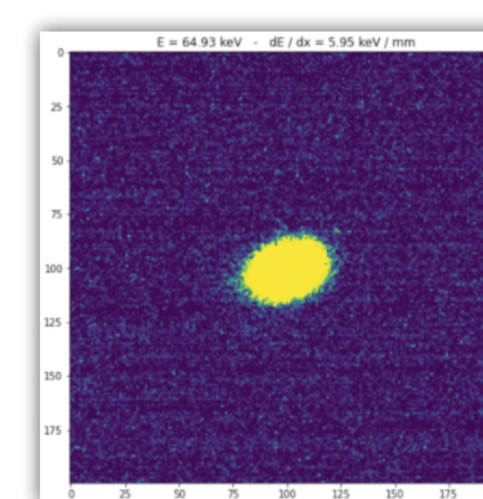
Light density and track shape strongly depend on the **particle energy** and identity
