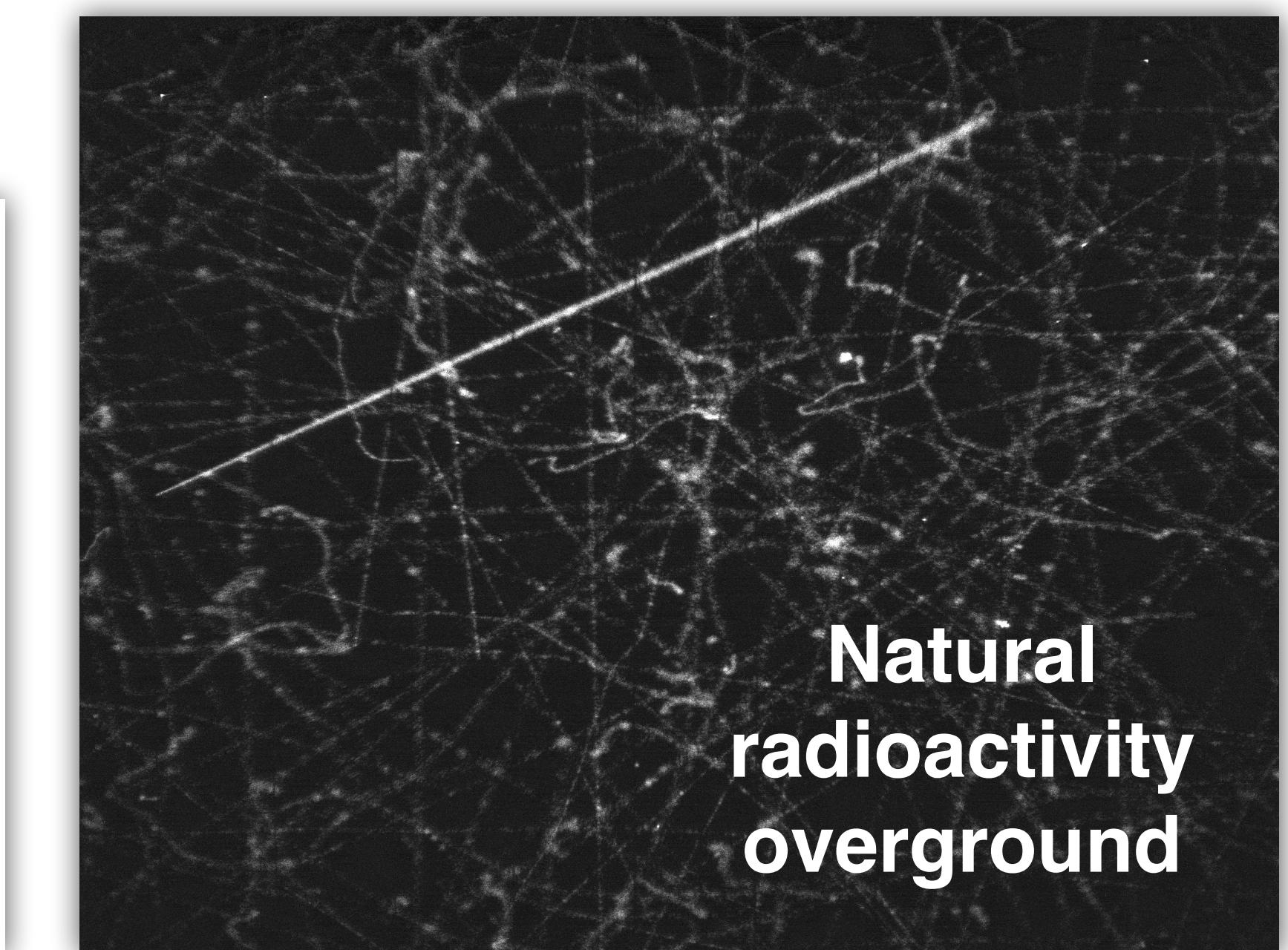
In the **avalanche processes** CF3\* created by electron dissociation and its de-excitation results in **light** **sCMOS** camera: single photon detection; high granularity and **XY reconstruction**
