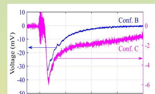
Oscilloscope waveforms read out from photodetector as a result of an X-ray pulse detected by using the detection unit in configurations with the wedge-shaped sample when only the forward transition of the probe beam with multiple reflections is employed (B), and with the wedge-
