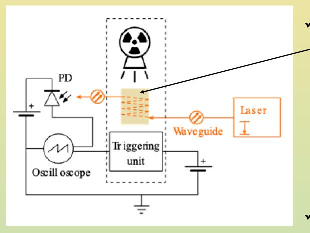
Outline of the system for detection of ionizing radiation based on radiationinduced optical absorption and remote readout  ✓ Gd<sub>3</sub>Al<sub>2</sub>GA<sub>3</sub>O<sub>12</sub>:Ce (GAGG:Ce) exhibited the best performance among other wide-band-gap semiconductors and scintillators tested (GaN, SiC, PbWO4 (PWO), Lu<sub>2</sub>SiO<sub>5</sub>:Ce (LSO:Ce), Y<sub>3</sub>Al<sub>5</sub>O<sub>12</sub>:Ce (YAG:Ce))
