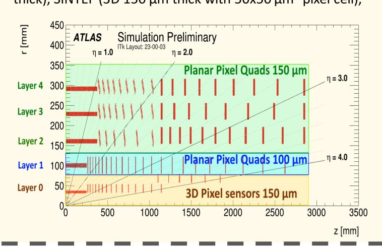
HPK (planar 150 μm thick) and FBK<sup>3</sup> (planar 100 μm thick and 3D 150  $\mu m$  thick with 25x100  $\mu m^2$  and 50x50  $\mu m^2$ pixel cell). In this poster, we present efficiency results of SINTEF 3D<sup>2</sup> and HPK planar<sup>1</sup> sensors. Such sensors were tested at fluences above 1.0x10<sup>16</sup> n<sub>eq</sub>/cm<sup>2</sup> (SINTEF 3D) and  $4.31 \times 10^{15} \, n_{eq}/cm^2$  (HPK planar).
