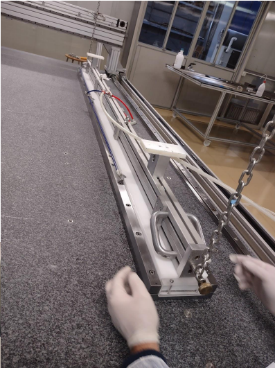
Stiffback-like technique for tube handling, gluing and positioning in the assembly tool
