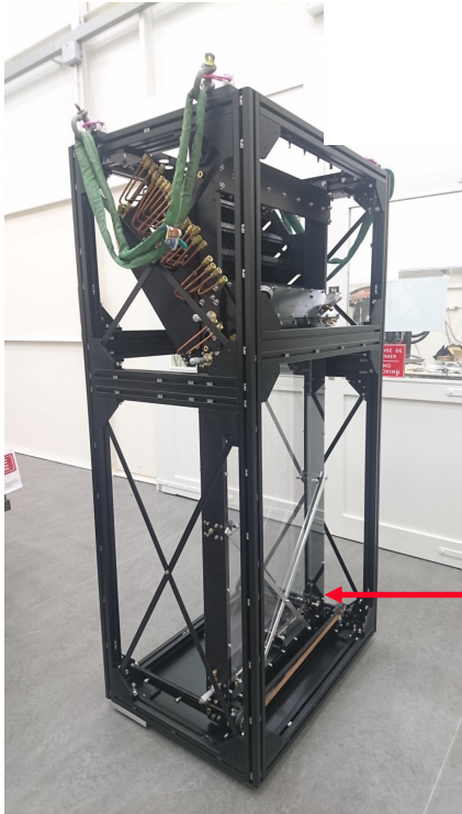
Full-scale half-length module with 1250 \times 660 \times 10 \text{ mm}^3 fused-silica radiator bar
