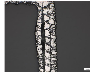
Pic05 – edge region. Decohesion of a built layer and pores are noticed Original magnification \times 100
