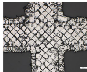
Pic02 – cross region. Microcrack in contouring layer and pores are noticed Original magnification \times 100
