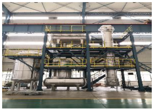
3) Water extraction to remove radioactive impurities
