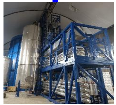
4) Gas stripping to remove Rn and O 2
