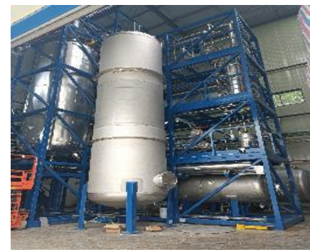
2) Distillation for radiopurity
