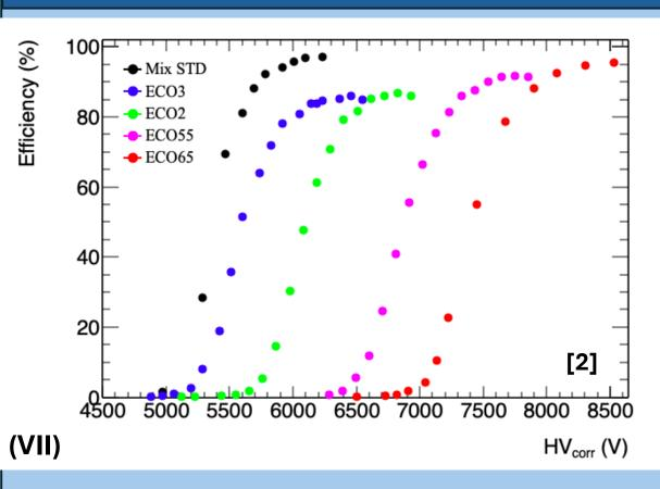
$C_3H_2F_4$  concentration above 50% (ECO55 and ECO65) is needed in order to achieve efficiency > 90%.
