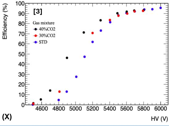
The gas mixtures containing  $CO_2$ achieve efficiency of 94%, 2% smaller than the standard gas (96%)
