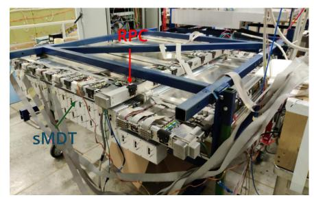
The most relevant innovations of the system lie in the reduced gas gap width and in the new FE electronics. The 1 mm gas gap width allows to lower the operating voltage (WP ~5.4 kV) and to improve the time resolution (0.4 ns) wrt the legacy 2 mm RPC (WP~ 9.6 kV, time resolution ~1 ns)
