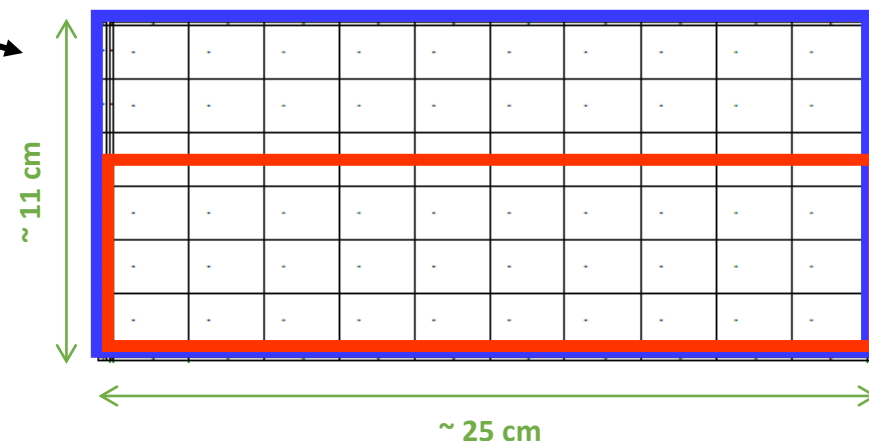
Allowed dimensions for stitched sensor on 30 cm wafer
