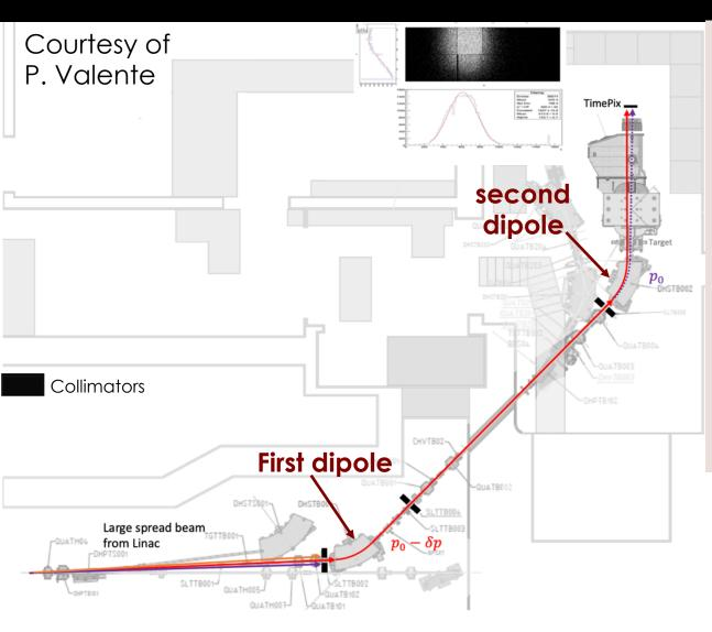
Use the first dipole magnet and collimators to select energy
