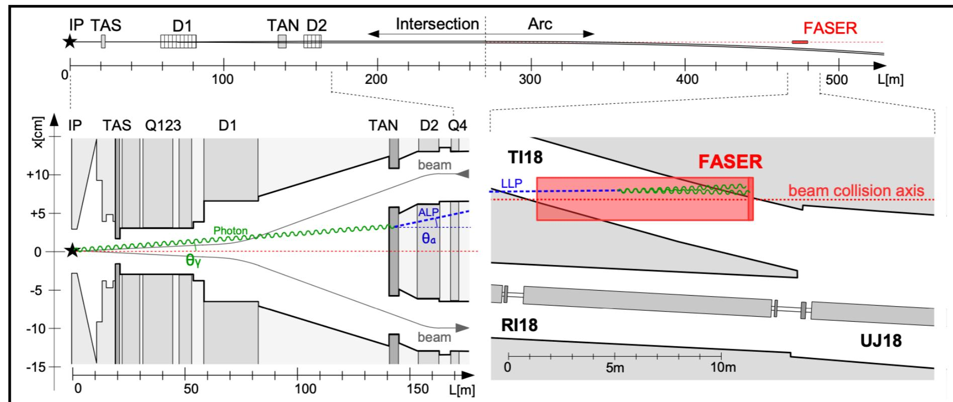
Exploits enormous forward cross-section at the LHC  $p p > \text{forward} \sim 100$  mb
