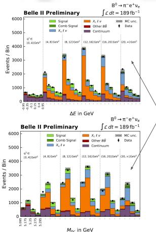
• Signal yields extracted in 6  $q^2$  bins by a 2D fit on energy difference  $\Delta E$  and beam-constrained mass  $M_{hc}$
