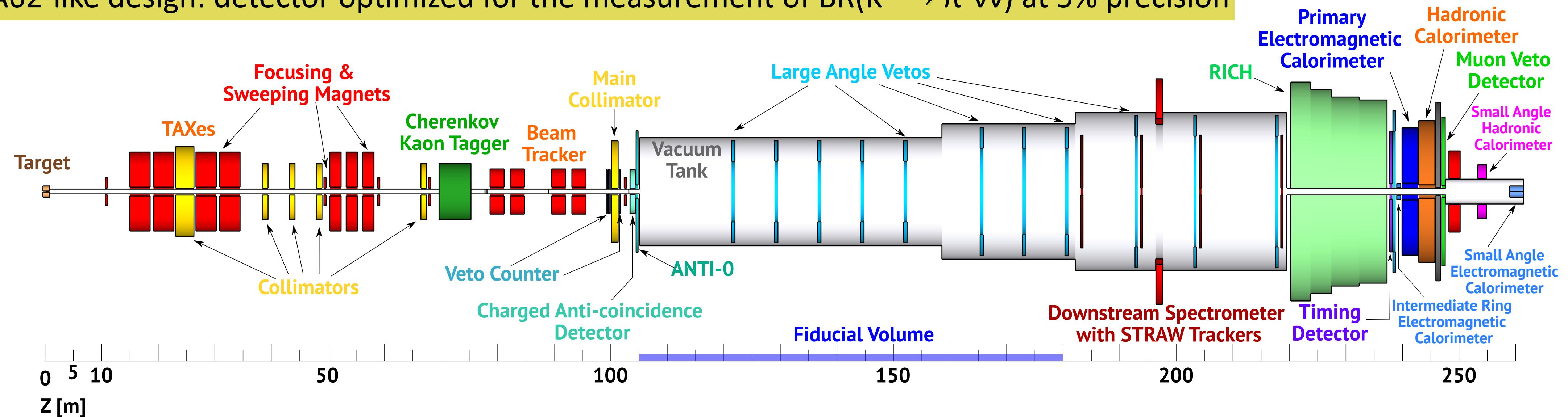
Full tracking of 3 GHz beam particle with 25 ps time resolution, tagging of 200 MHz  $\text{K}^+$  and high-rate precision tracking of secondary particles
