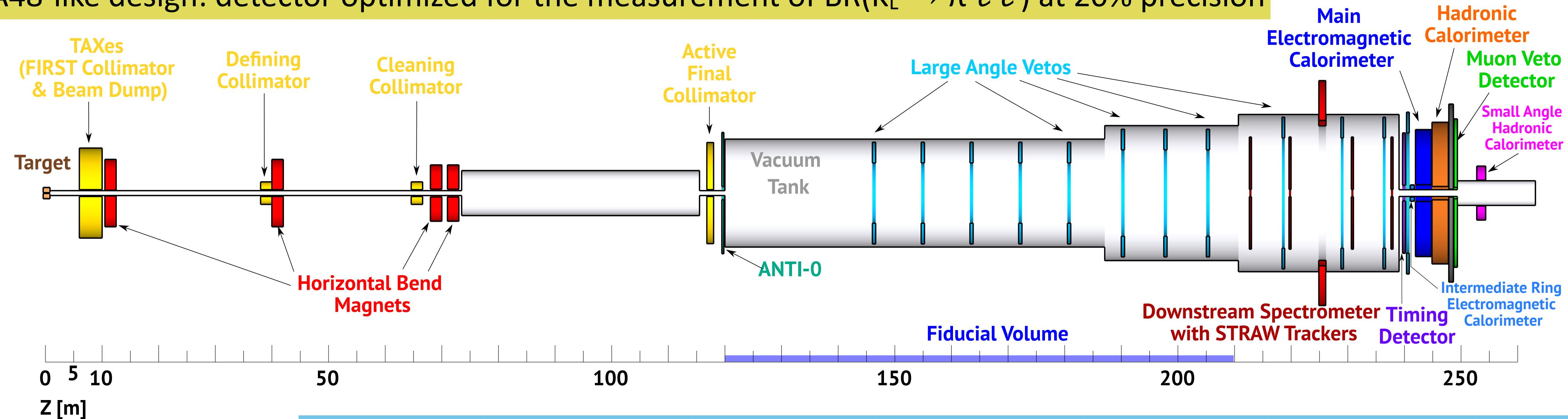
Challenges: 90m long instrumented decay volume, 100 ps time resolution for  $\pi^0$  of few GeV energies
