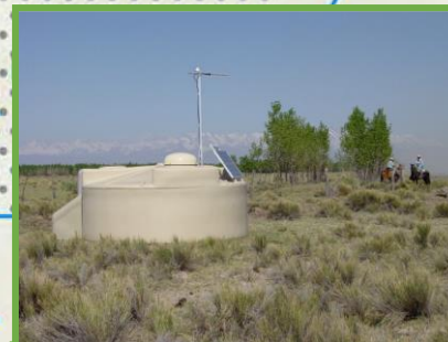
1665 surface detectors: water-Cherenkov tanks (grid of 1.5 km, 3000 km 2 )
