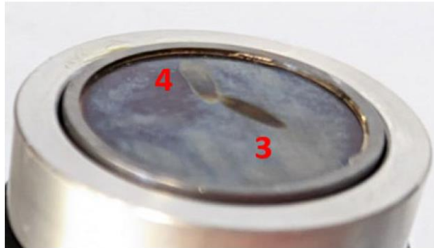
Fig. 3. Beryllium-vanadium target after irradiation. Beam spot (3) and (4) correspond to the run with surface power density of 600 and 400 W/cm 2 , respectively. In both cases, no macroscopic blistering is visible.
