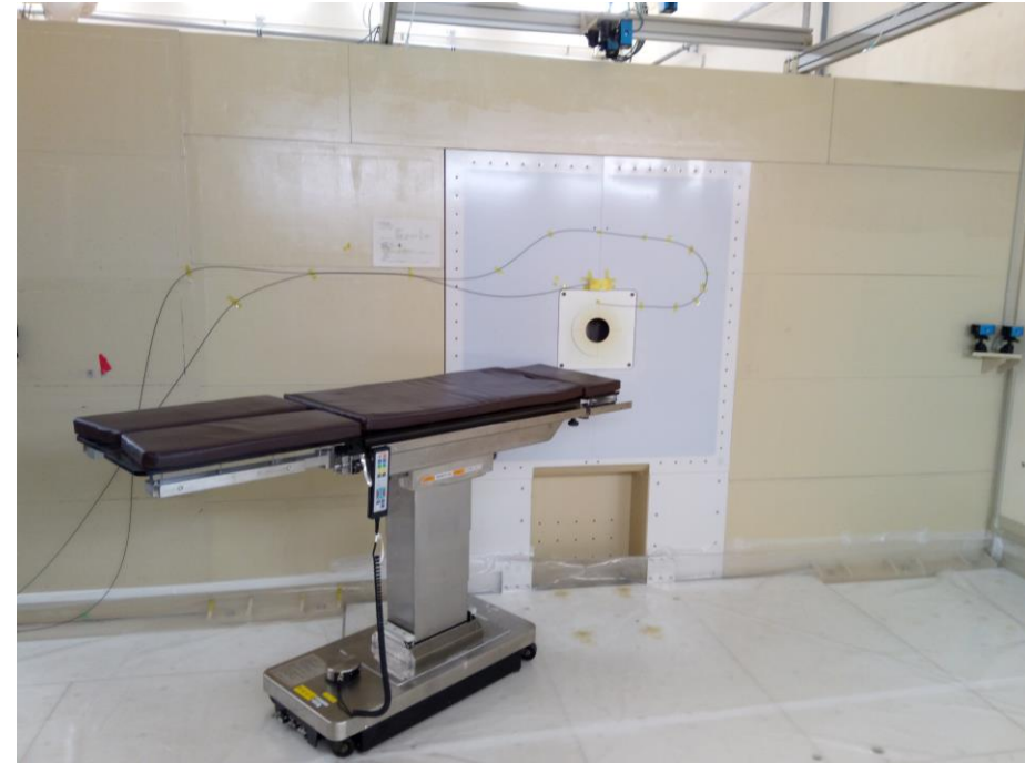
Beryllium target assembly and treatment bed at iBNCT
