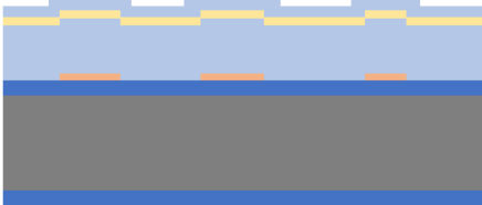
2- PECVD oxide (5 um) and protective mask (Al/PECVD oxide)
