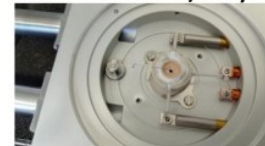
cell for HT Raman/x-ray expts
