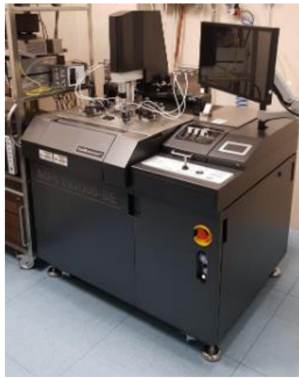
Test done on MPI PA200 Test Station in the Clean Room. Thanks to CMS group: A. Rossi, F. Moscatelli
