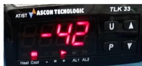
Temperature at coldbox4-vacuum (pt100)
