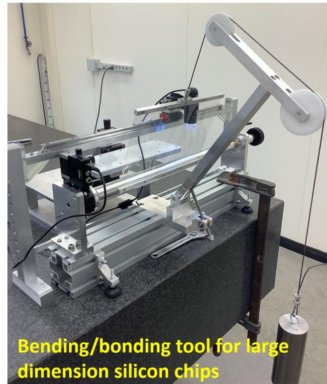
Bending/bonding tool for large dimension silicon chips
