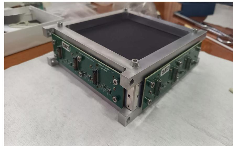
The readout PCB hosting SiPM
