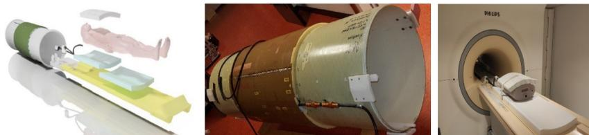
Figure 1. The schematic overview of the metabolic MRI setup (left) including the embedded double-tuned body transmitter (middle) and the wrap-around transceiver and receiver array for <sup>1</sup>H, <sup>2</sup>H and <sup>31</sup>P MRI.
